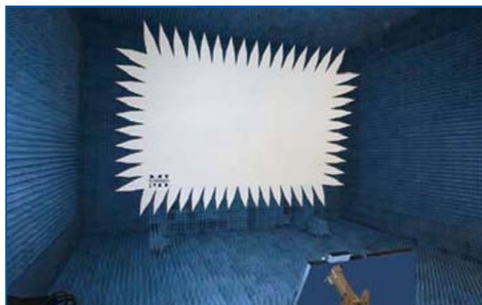
Figure 2: Compact Range Reflector and Feed located at the Instituto Nacional de Tecnica Aeroespacial (INTA) in Spain. This CR is capable of testing the RCS of objects up to 5.5 meters wide by 5 meters tall.
