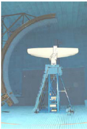
Fig.6, A Spherical NF Arch with Utility Radar From BAE Systems, Isle of Wight, UK
