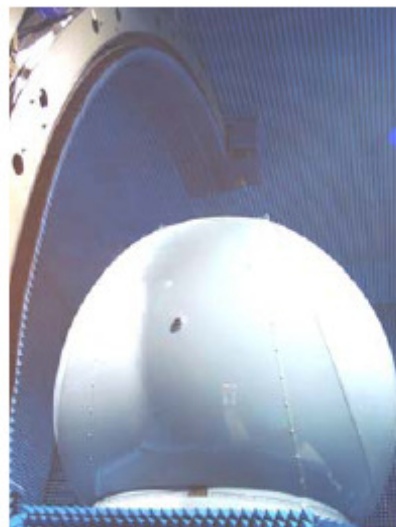
Fig.7, Spherical NF Arch with Sampson Radome From BAE Systems, Isle of Wight, UK
