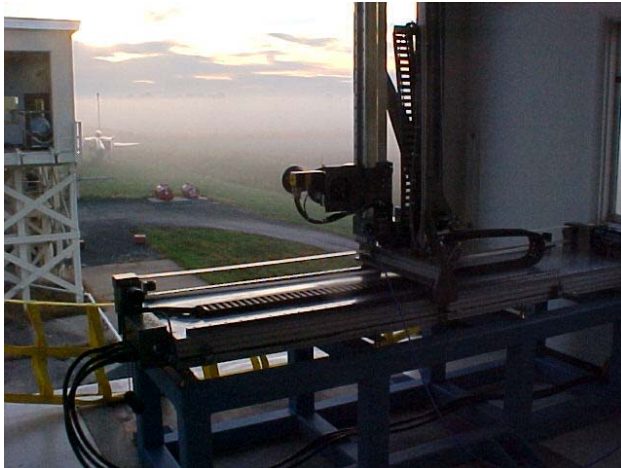
Figure 4. MI-3630 5x5 Ft. X-Y Scanner
