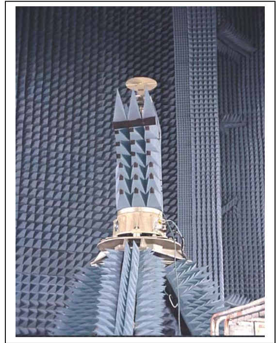
Fig. 10. A Small 18 in diameter Flat Plate Array Mounted on the Spherical Near-Field Scanner Close to the Point of Axis Intersection
