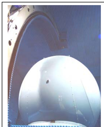
Fig.16, Spherical NF Arch with Sampson Radome From BAE Systems Insyte, Isle of Wight, UK
