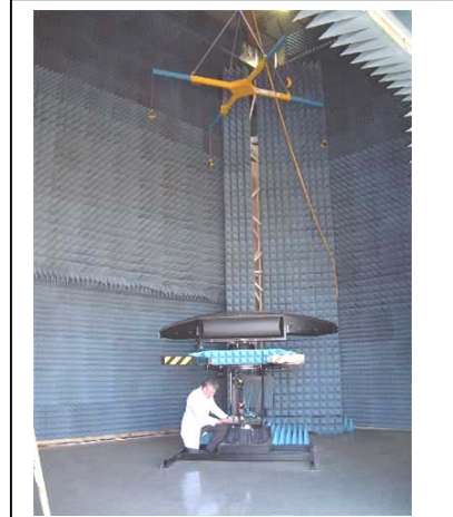
Fig.14, A 6 m Cylindrical NF Range Courtesy C.McCartney, Chelton Composites
