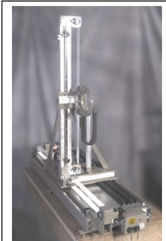
Fig.5, An x-y Positioner Used as Null Seeker
