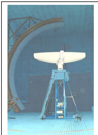
Fig.15, A Spherical NF Arch with Utility Radar From BAE Systems Insyte, Isle of Wight, UK
