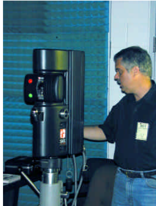
Figure 4: The SMX Model 4000 Tracking Laser Interferometer and John Proctor from MI Technologies.
