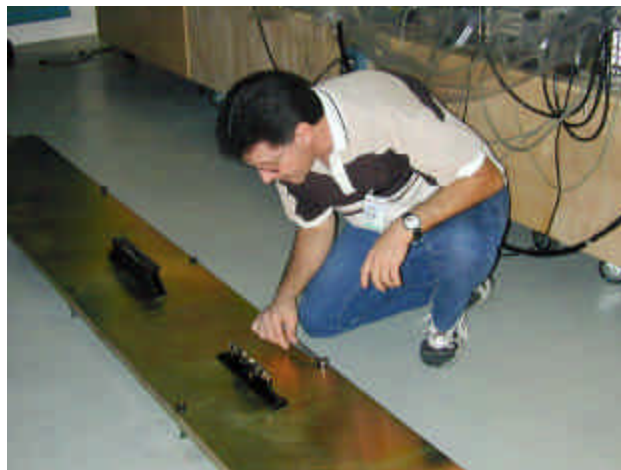
Figure 2: Carlos Turano is working on the first step of the scanner alignment by making the base plate level.
